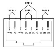
Figure 6-2. RJ-45 connector using T568B wiring.
